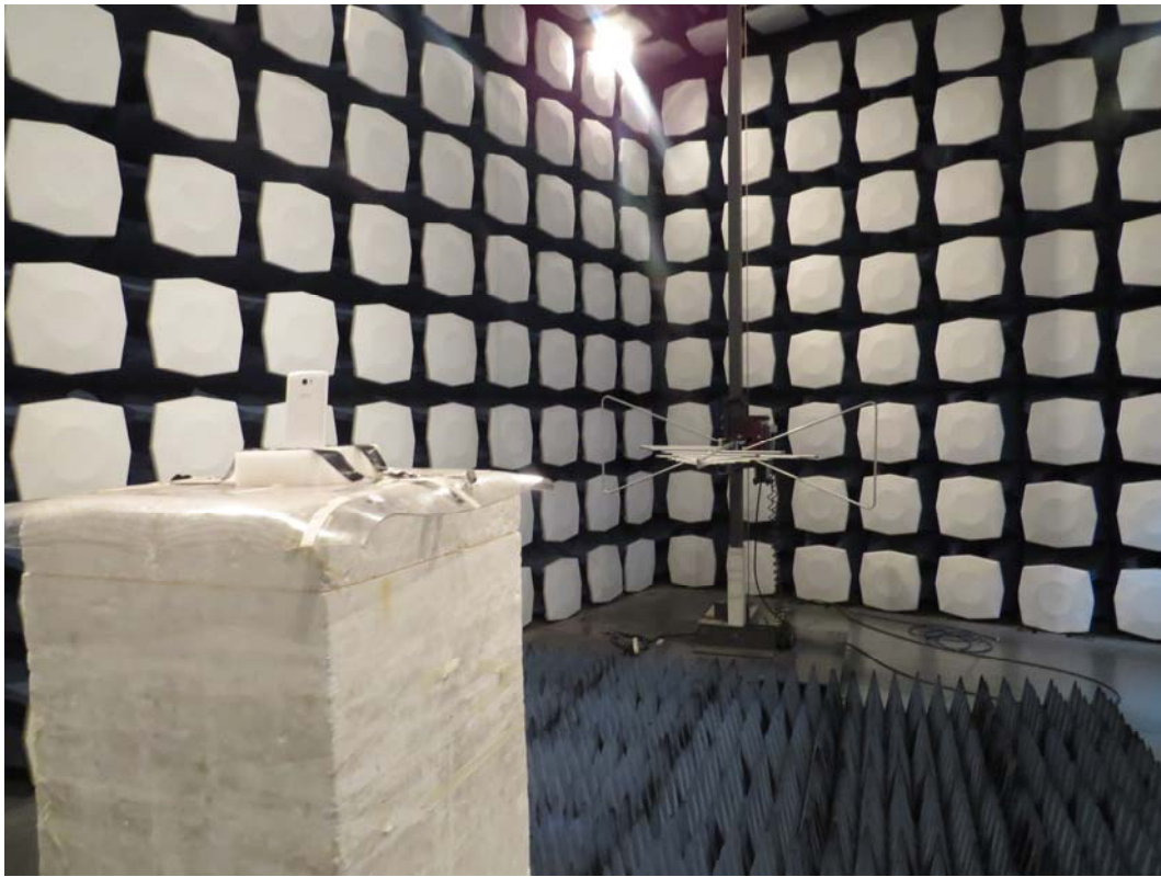
Picture 2: Radiated Spurious Emissions Test setup
