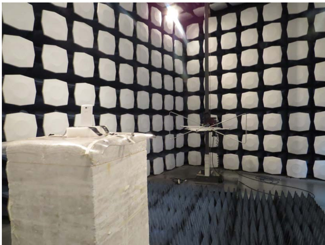
Picture 2: Radiated Spurious Emissions Test setup
