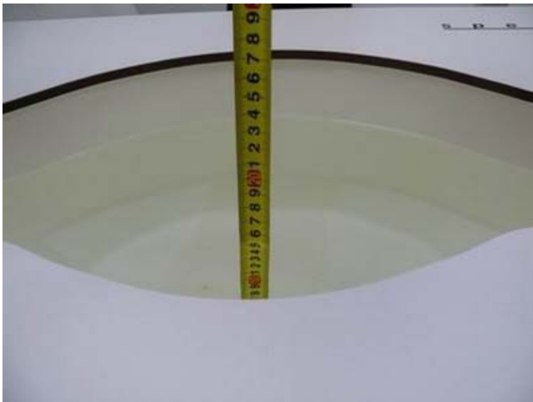
Picture 7: Liquid depth in the flat Phantom (1900 MHz, 15.2cm depth)
