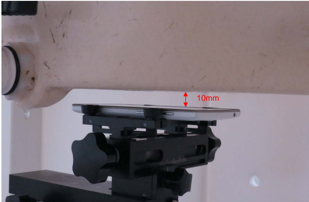
Front Side, the distance from handset to the bottom of the Phantom is 10mm
