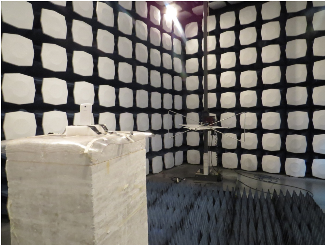
Radiated Spurious Emissions Test setup
