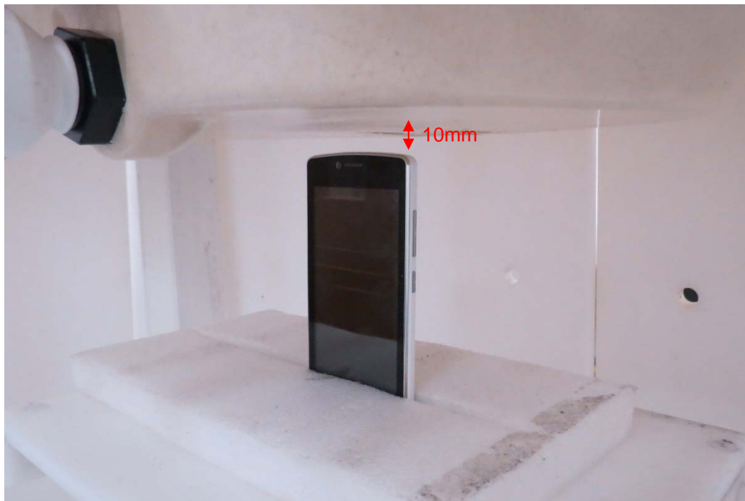
Top Side, the distance from handset to the bottom of the Phantom is 10mm
