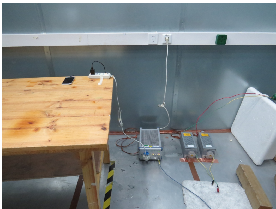
Conducted Emission Test Setup
