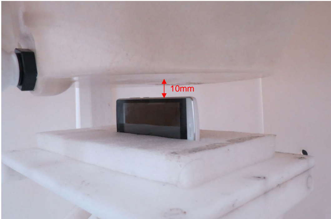
Right Side, the distance from handset to the bottom of the Phantom is 10mm
