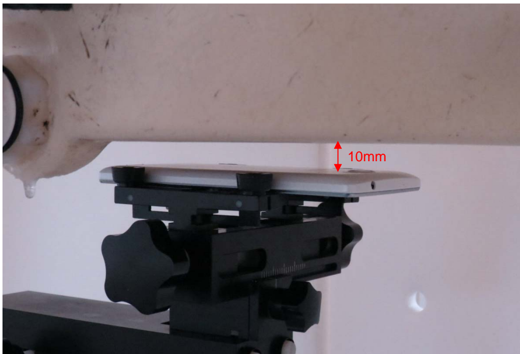
Back Side, the distance from handset to the bottom of the Phantom is 10mm
