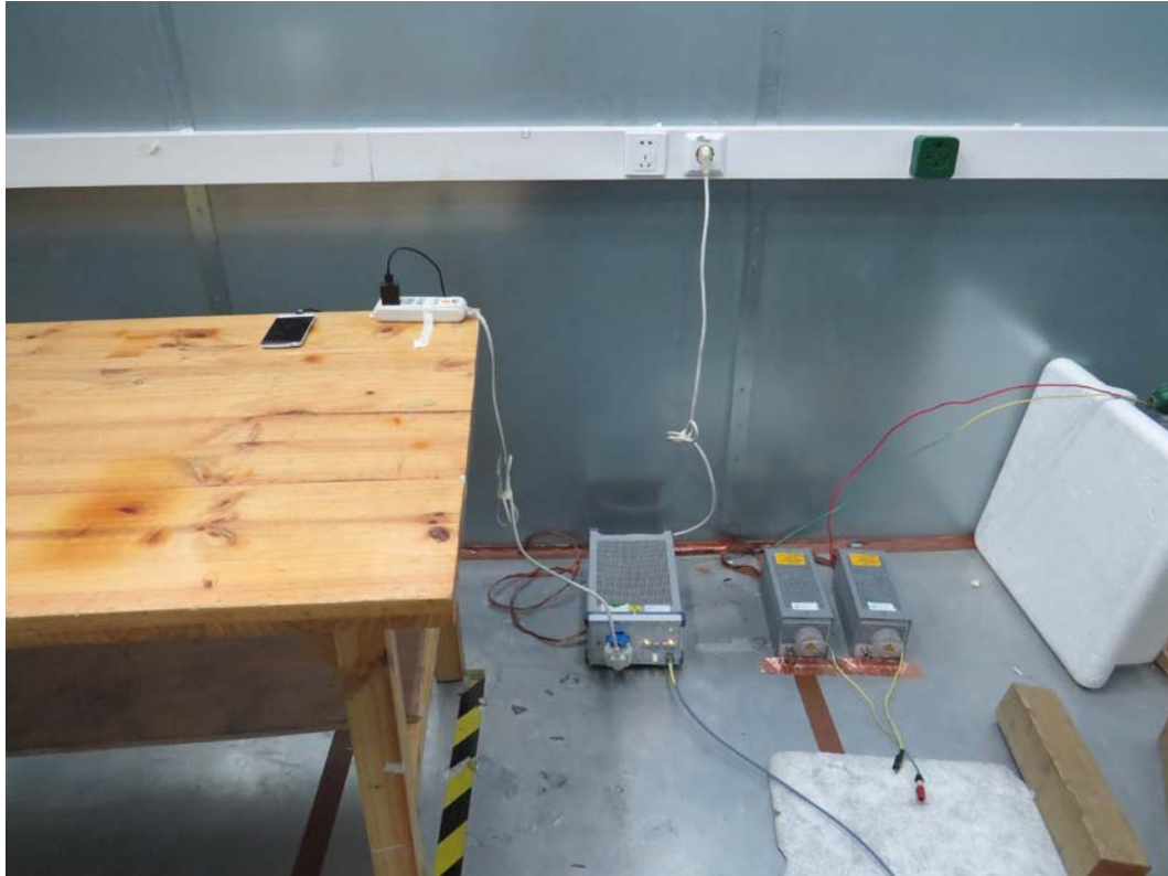
Picture 3 Conducted Emission Test Setup
