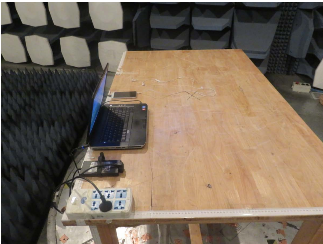
Picture 2 Radiated Emission Test Setup
