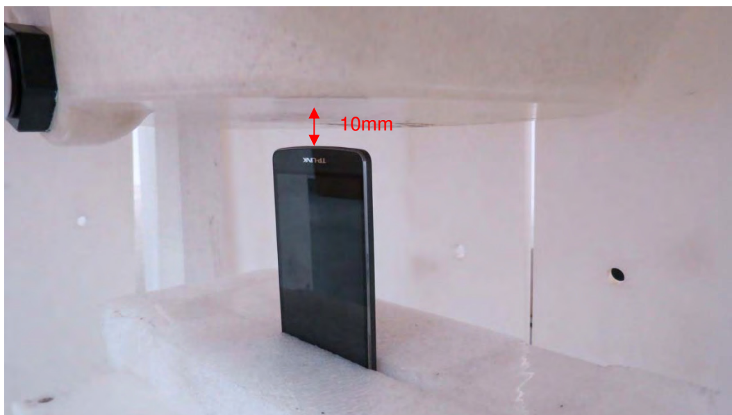
Picture 23: Bottom Side, the distance from handset to the bottom of the Phantom is 10mm
