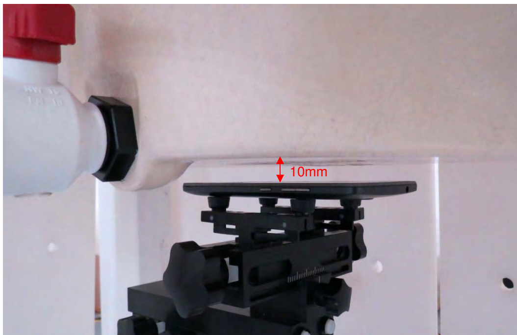
Picture 19: Front Side, the distance from handset to the bottom of the Phantom is 10mm
