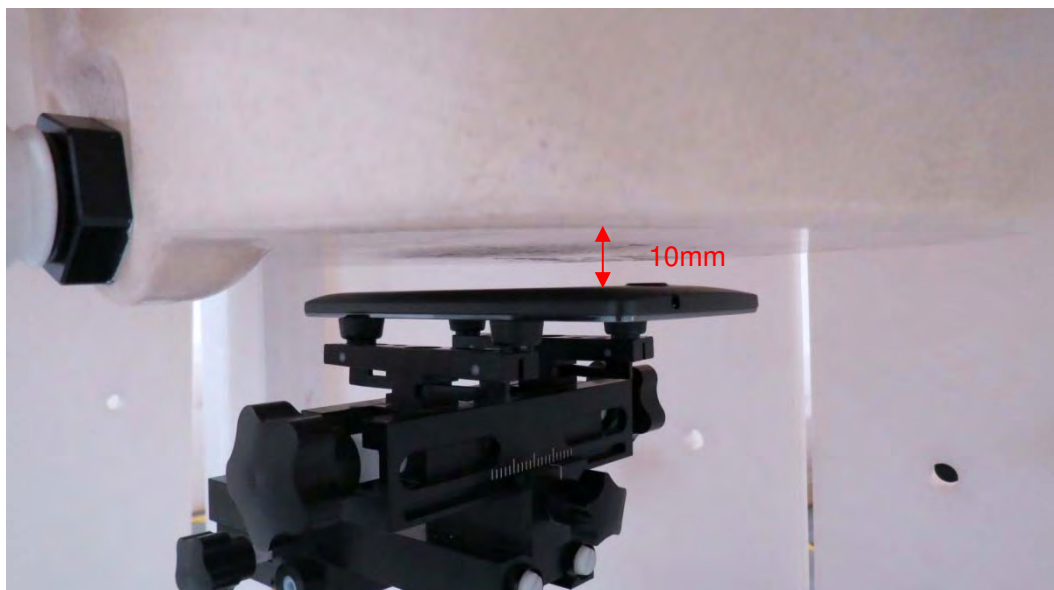
Picture 18: Back Side, the distance from handset to the bottom of the Phantom is 10mm
