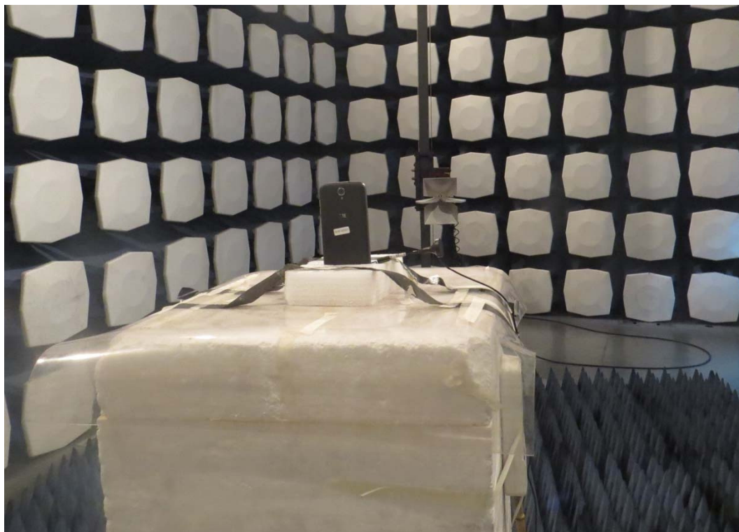
Picture 2 Radiated Spurious Emissions Test Setup
