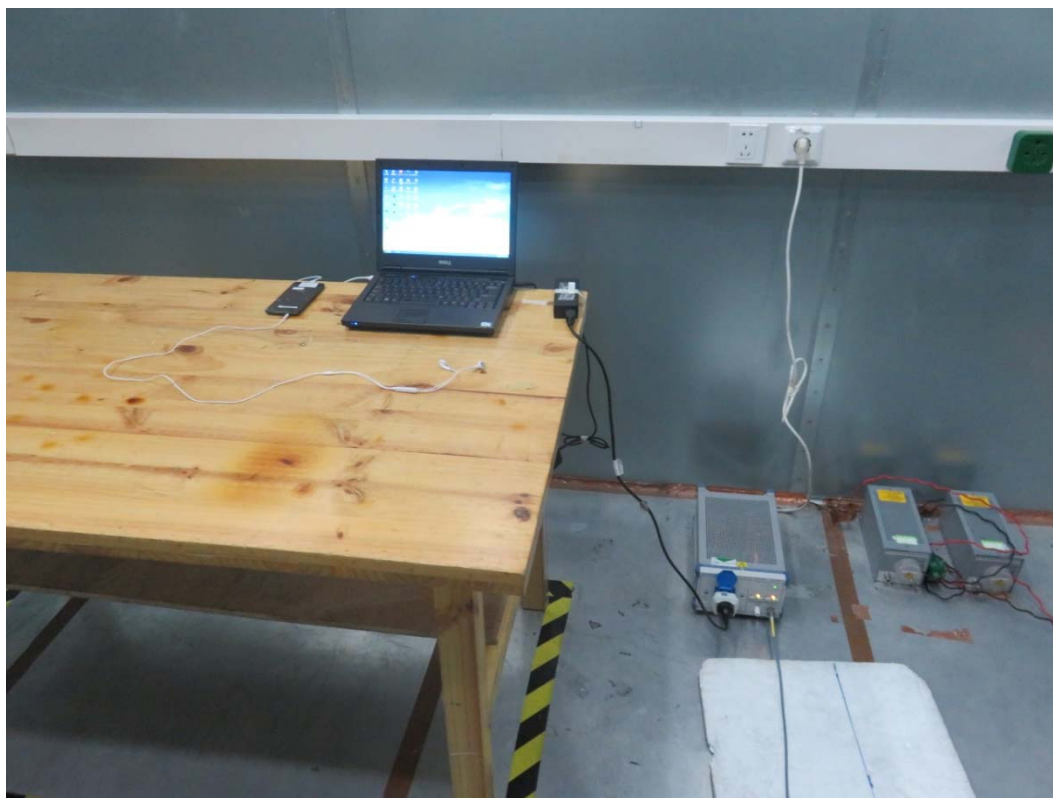
Picture 2 Conducted Emission Test Setup
