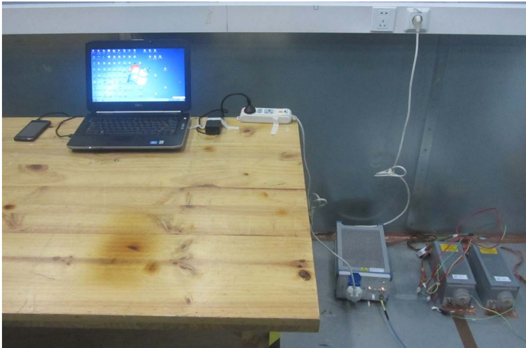
Picture 3 Conducted Emission Test Setup
