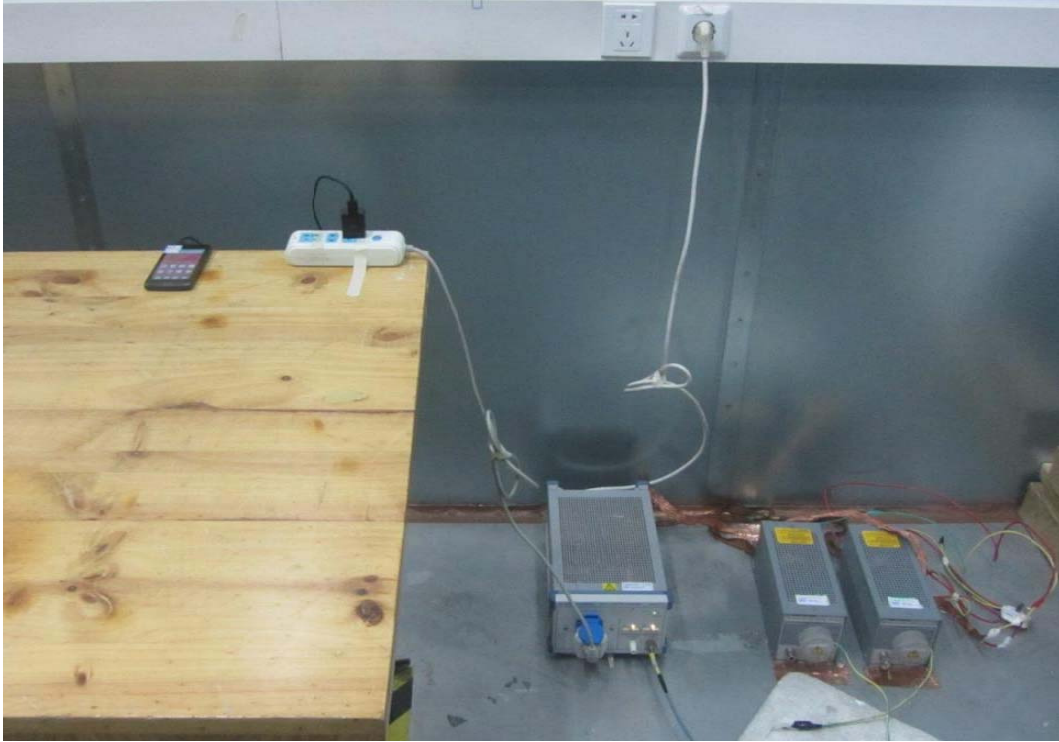
Picture 3 Conducted Emission Test Setup
