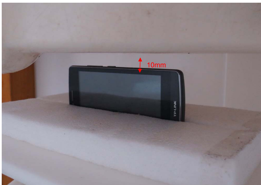
Picture 21: Right Side, the distance from handset to the bottom of the Phantom is 10mm
