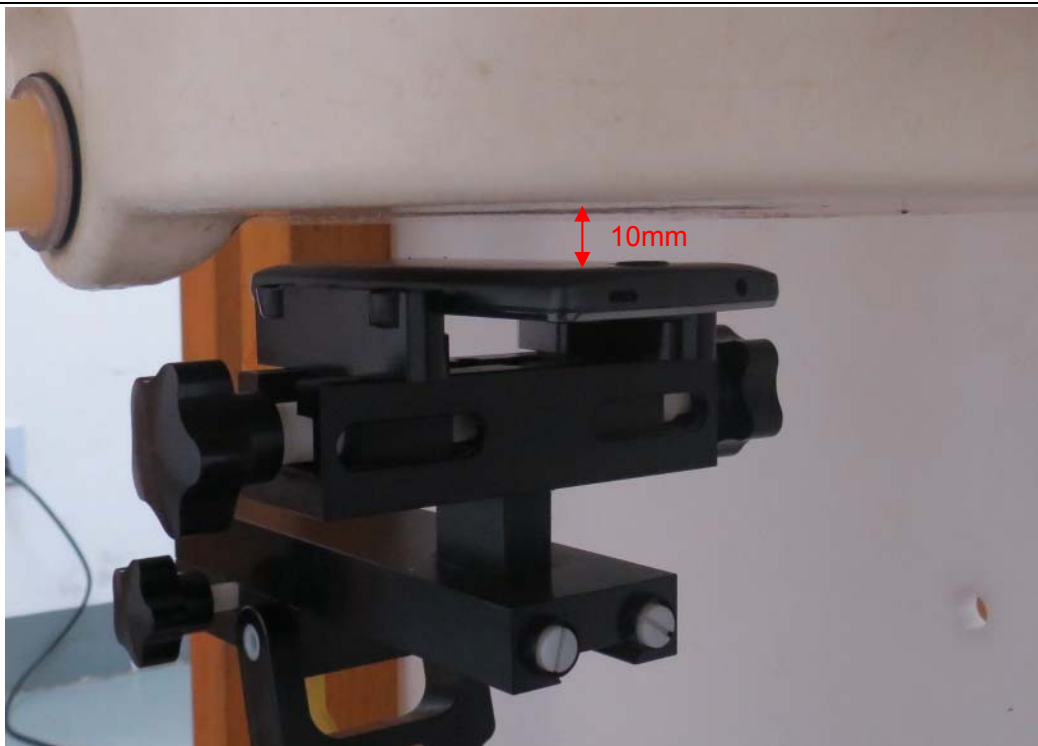
Picture 18: Back Side, the distance from handset to the bottom of the Phantom is 10mm
