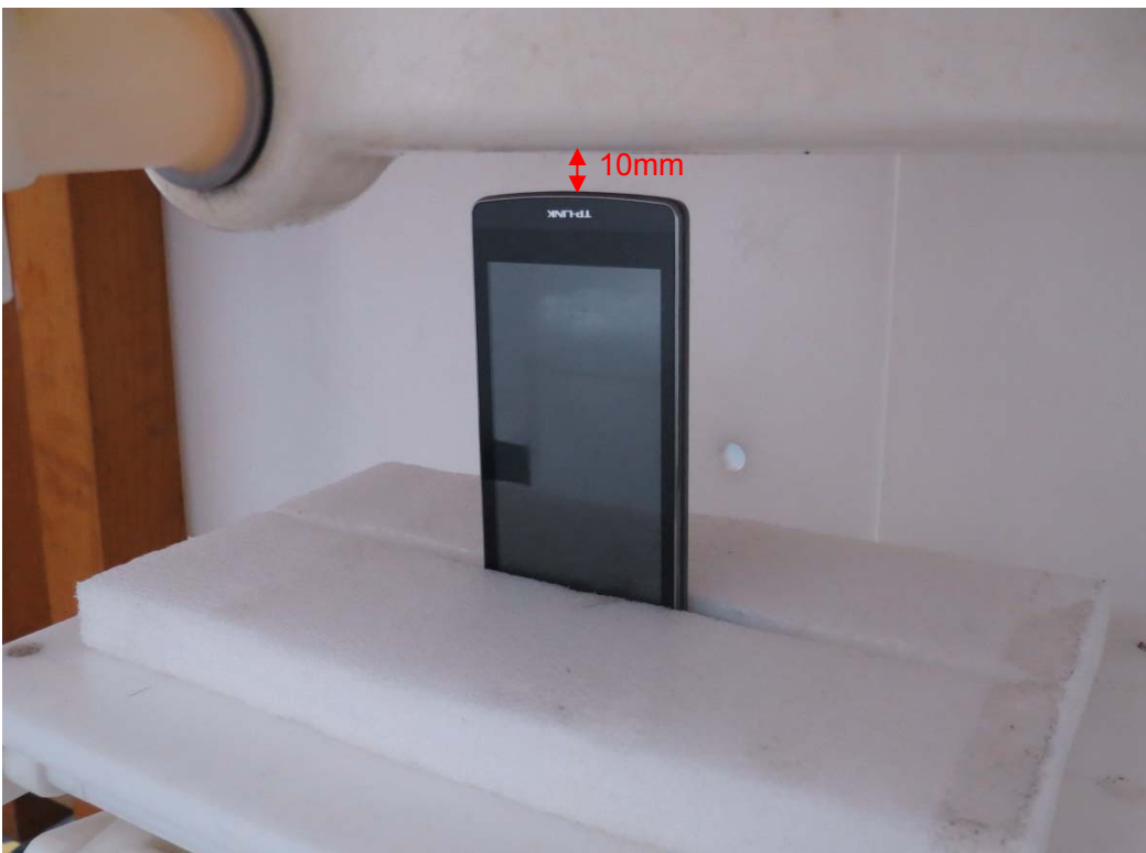
Picture 23: Bottom Side, the distance from handset to the bottom of the Phantom is 10mm
