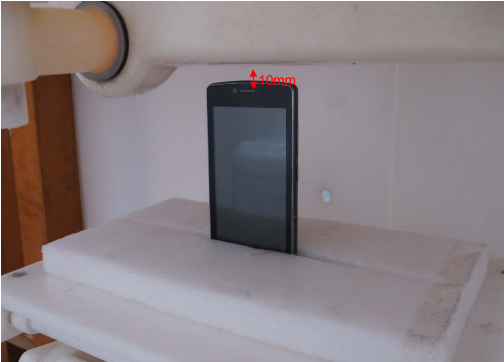
Picture 22: Top Side, the distance from handset to the bottom of the Phantom is 10mm
