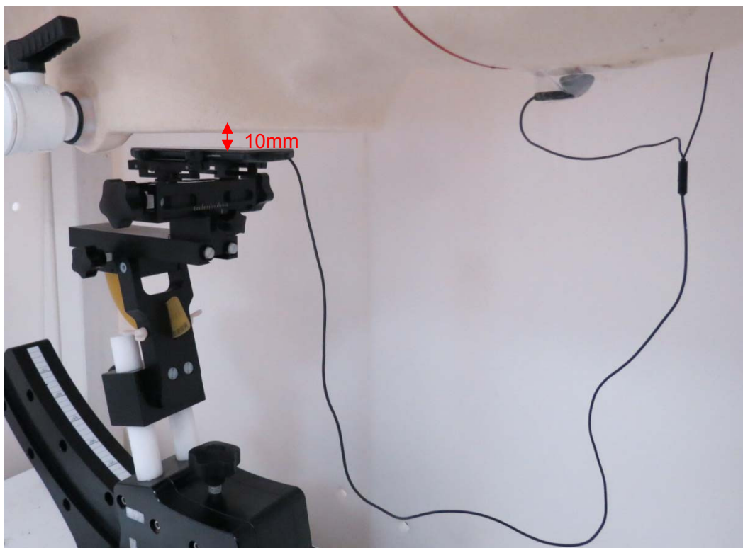
Picture 25: Front Side with Earphone, the distance from handset to the bottom of the Phantom is 10mm
