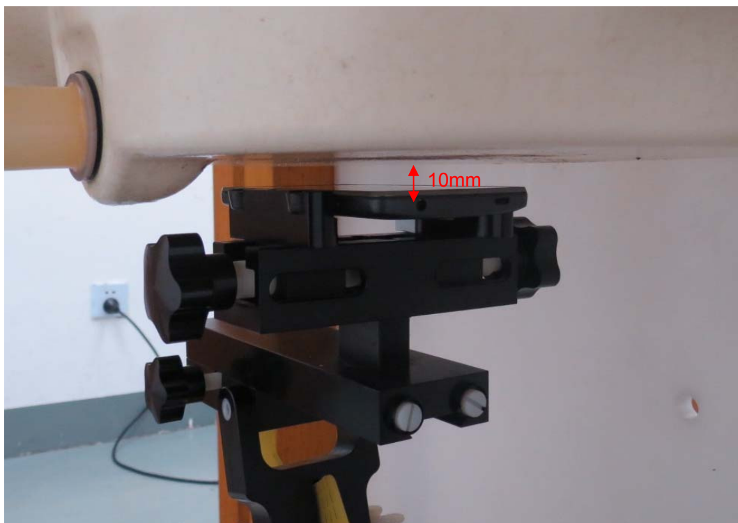
Picture 19: Front Side, the distance from handset to the bottom of the Phantom is 10mm
