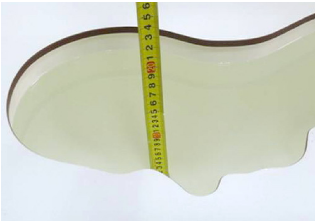
Picture 10: Liquid depth in the head Phantom (2450 MHz, 15.4cm depth)
