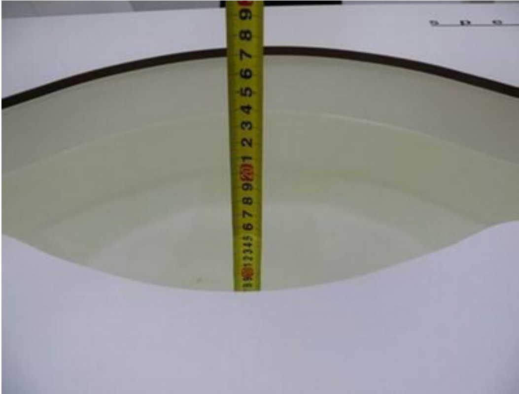
Picture 9: Liquid depth in the flat Phantom (2450 MHz, 15.3cm depth)
