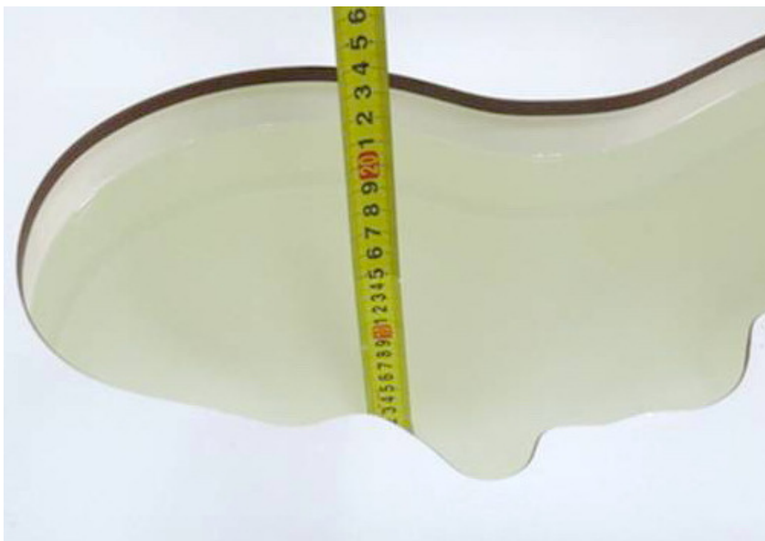
Picture 12: Liquid depth in the head Phantom (2600 MHz, 15.4cm depth)
