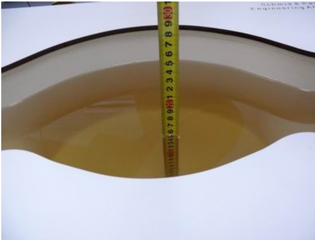
Picture 3: Liquid depth in the flat Phantom (835MHz, 15.4cm depth)
