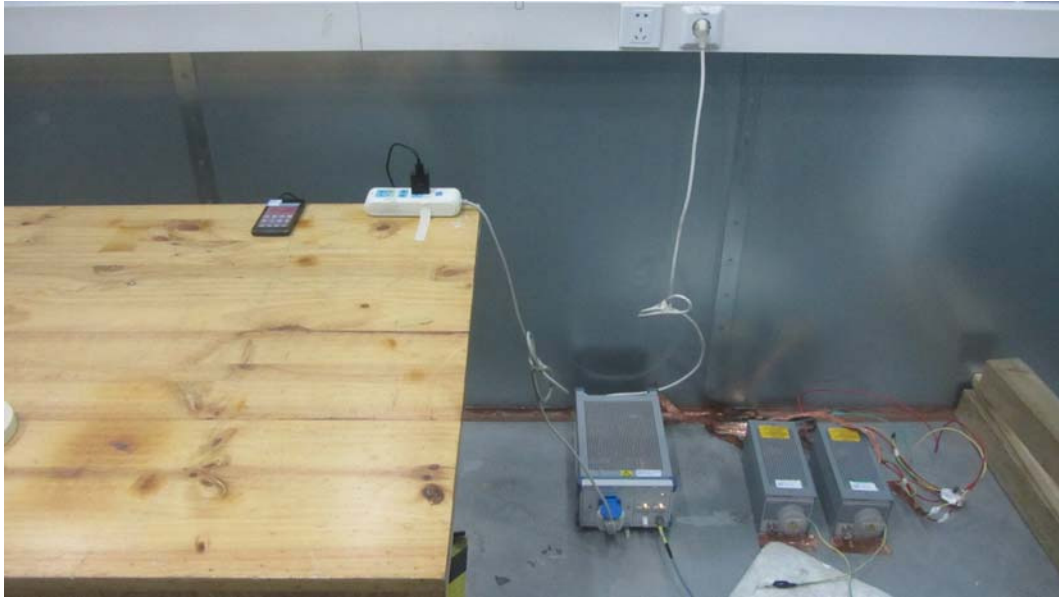
Picture 3 Conducted Emission Test Setup
