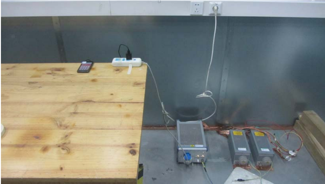
Picture 3 Conducted Emission Test Setup
