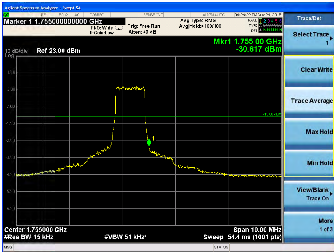
LTE Band 4 QPSK Bandwidth = 1.4MHz CH20393, RB 6
