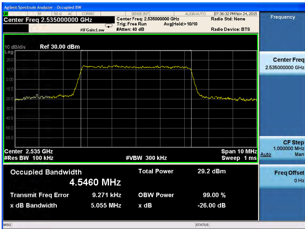
LTE Band 7 16QAM Bandwidth = 5MHz CH21100 Occupied Bandwidth
