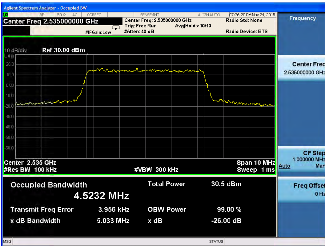
LTE Band 7 QPSK Bandwidth = 5MHz CH21100 Occupied Bandwidth
