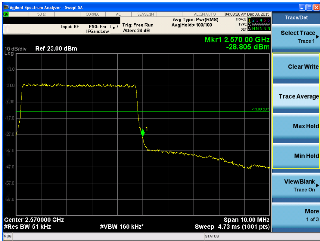
LTE Band 7 QPSK Bandwidth = 5MHz CH21425, RB 25
