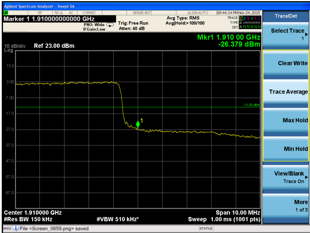
LTE Band II 15MHz 16QAM 100%RB CH19125
