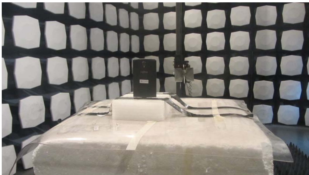
Picture 2: Radiated Spurious Emissions Test setup
