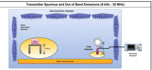
Magnetic field tests shall be performed in the frequency range of 9 kHz to 30 MHz using a calibrated loop antenna.
