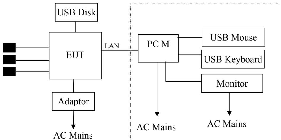
(EUT: AC750 Wireless Dual Band Gigabit Router)
