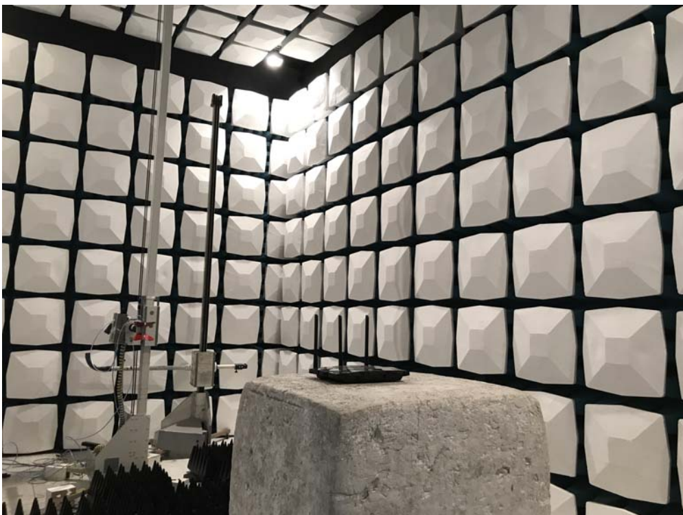
Description: Radiated Emission Test Setup for 1~18GHz
