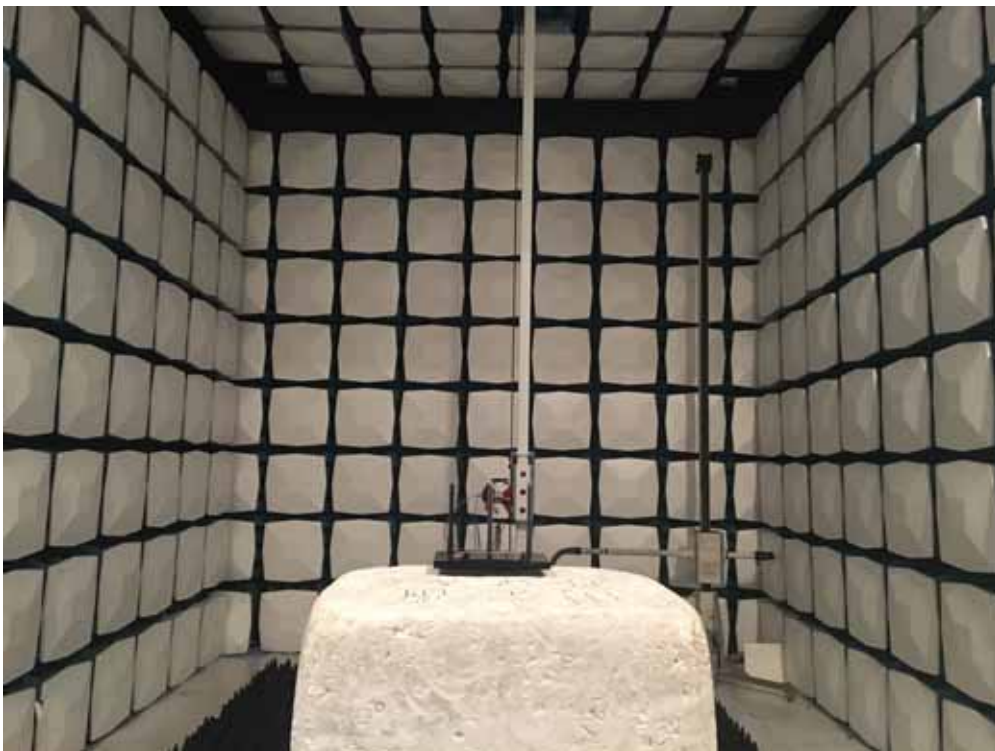
Description: Radiated Emission Test Setup for 1~18GHz
