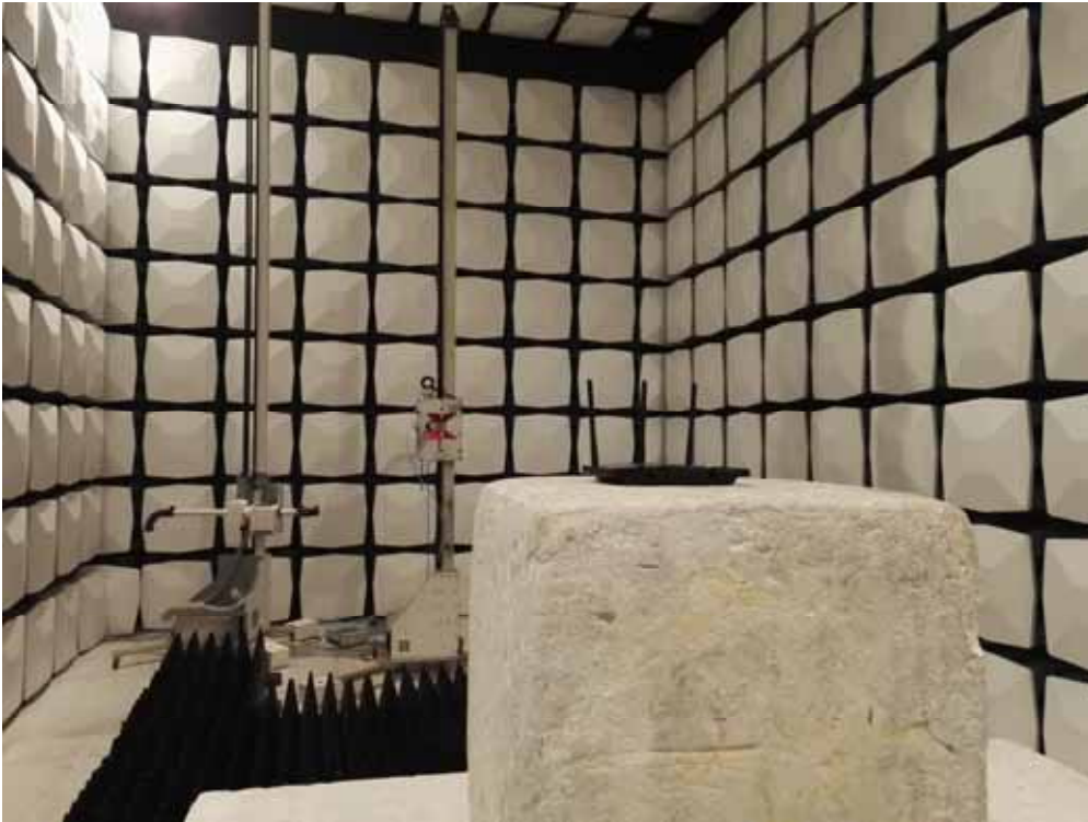
Description: Radiated Emission Test Setup for 1~18GHz
