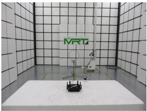
Description: Radiated Spurious Emission Test Setup for  $9kHz \sim 30MHz$
