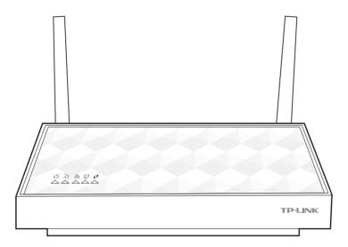
The AP device's LEDs are located on the top panel. You can check the AP device's working status by following the LED Explanation table (view from left to right).
