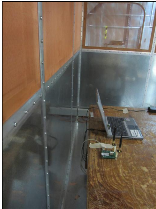
Photograph 2. Conducted Emissions, Test Setup, Side View
