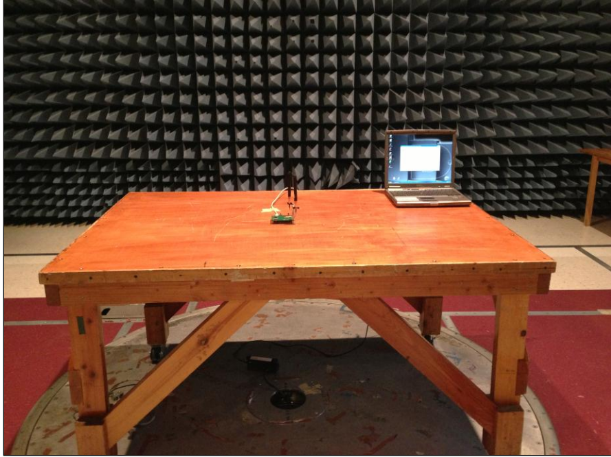
Photograph 3. Radiated Emissions, Test Setup
