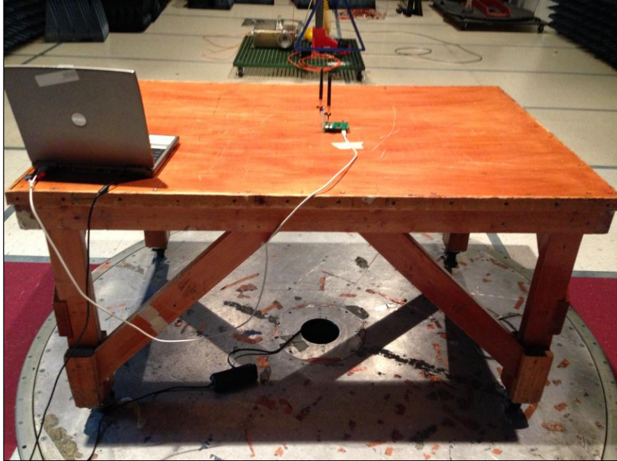
Photograph 5. Radiated Emissions, Test Setup, Rear View
