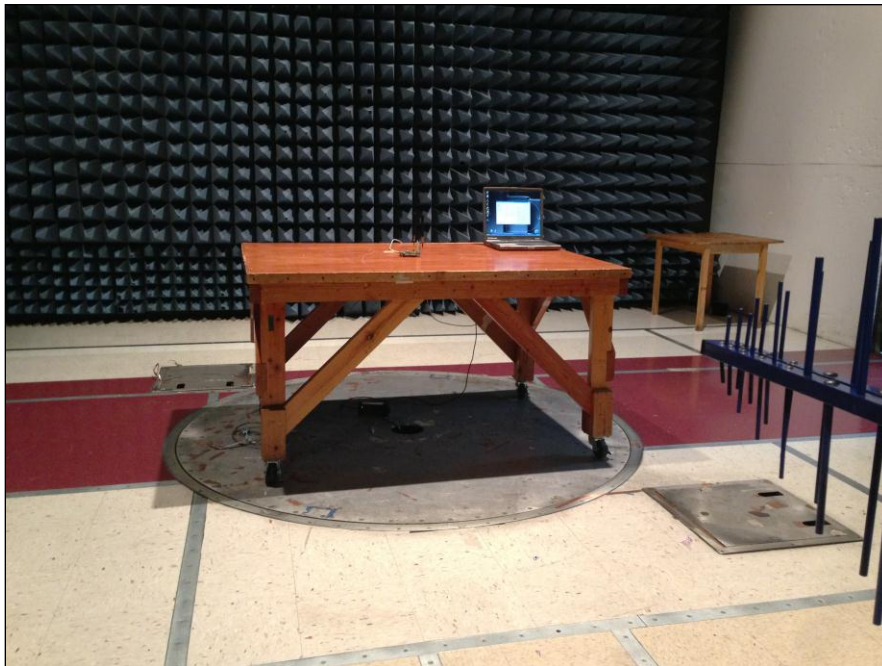
Photograph 10. Radiated Spurious Emissions, Test Setup, 30 MHz – 1 GHz
