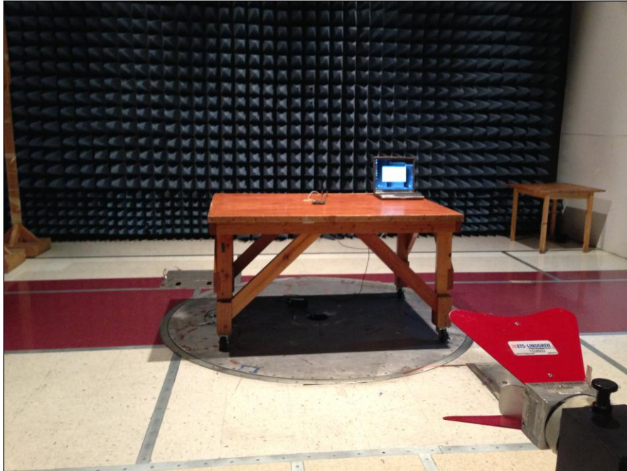
Photograph 9. Radiated Spurious Emissions, Test Setup, 3 m
