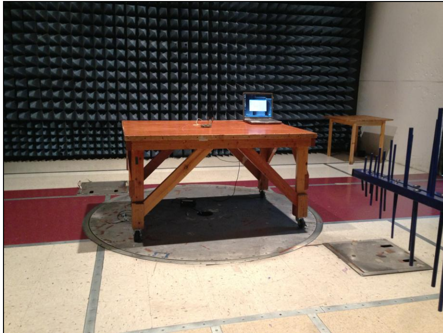
Photograph 11. Radiated Spurious Emissions, Test Setup, 30 MHz – 1 GHz
