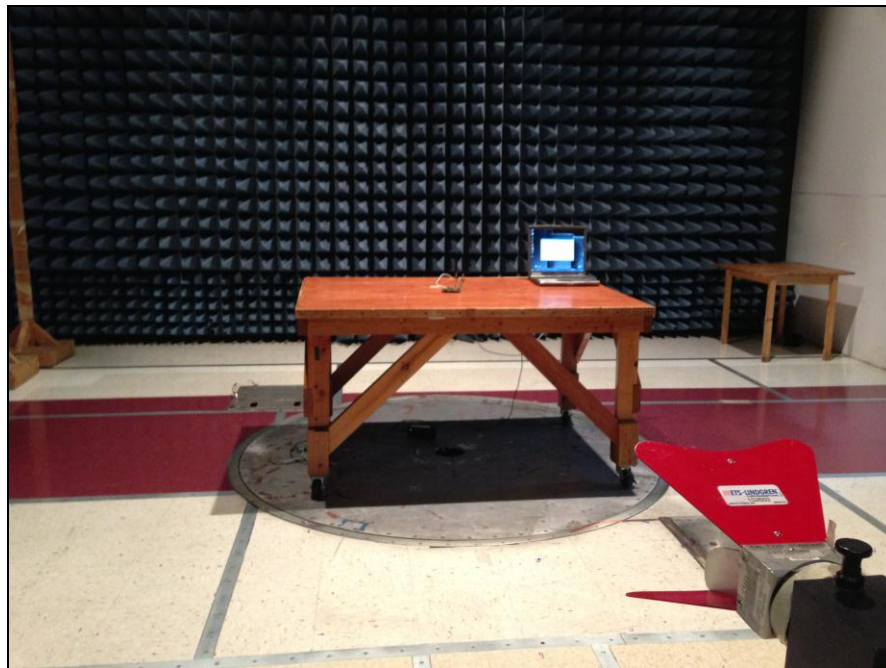
Photograph 10. Radiated Spurious Emissions, Test Setup, 3 m
