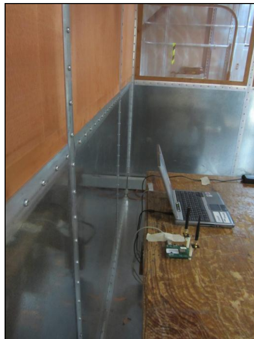
Photograph 8. Conducted Emissions, 15.207(a), Test Setup, Side View
