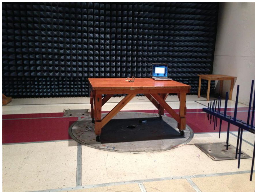
Photograph 5. Radiated Emissions, Test Setup, 30 MHz – 1 GHz
