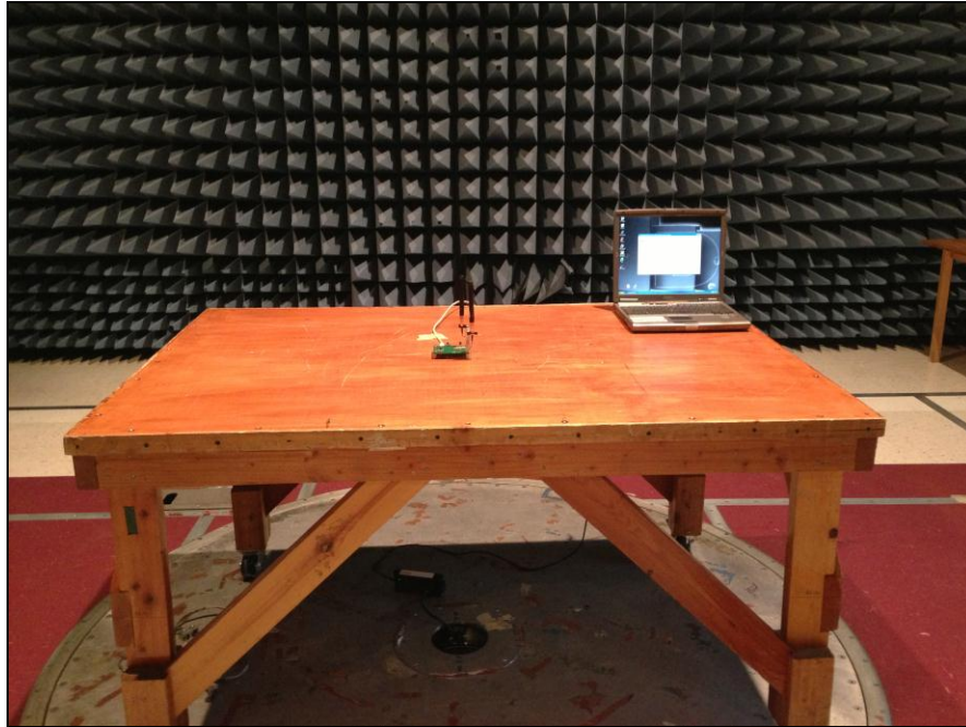
Photograph 4. Radiated Emissions, Test Setup
