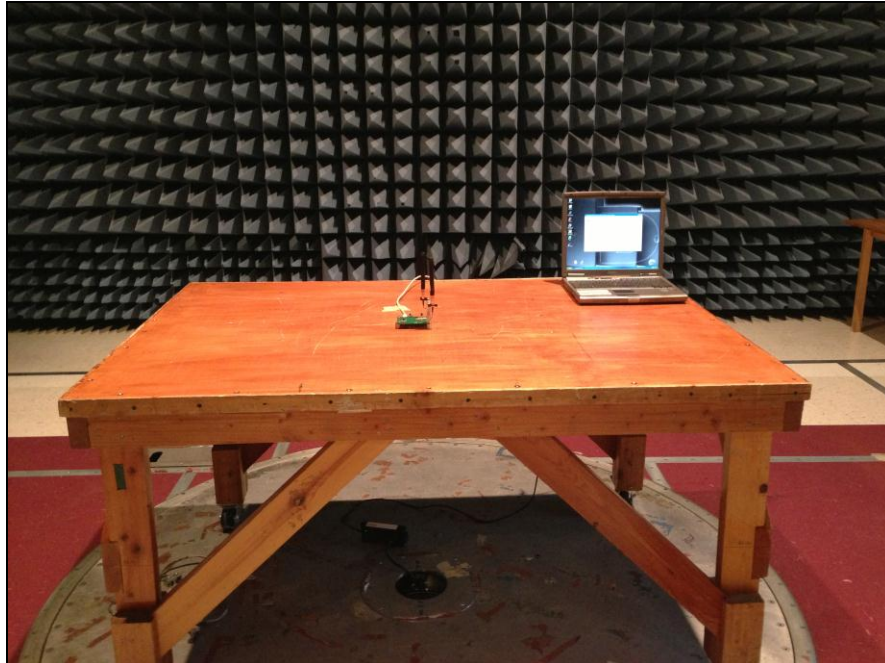
Photograph 12. Radiated Spurious Emissions, Test Setup
