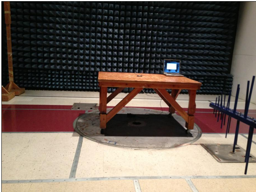
Photograph 4. Radiated Emissions, Test Setup, 30 MHz – 1 GHz
