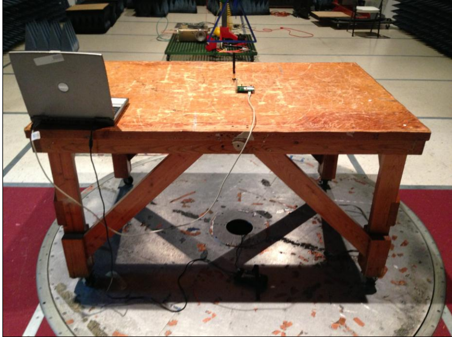
Photograph 5. Radiated Emissions, Test Setup, Rear View
