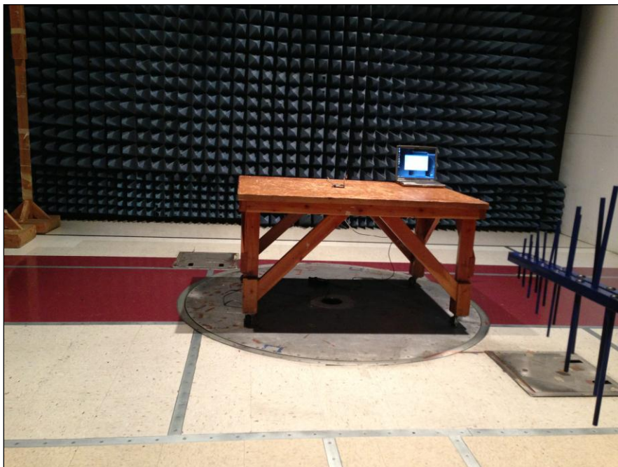
Photograph 10. Radiated Spurious Emissions, Test Setup, 30 MHz – 1 GHz
