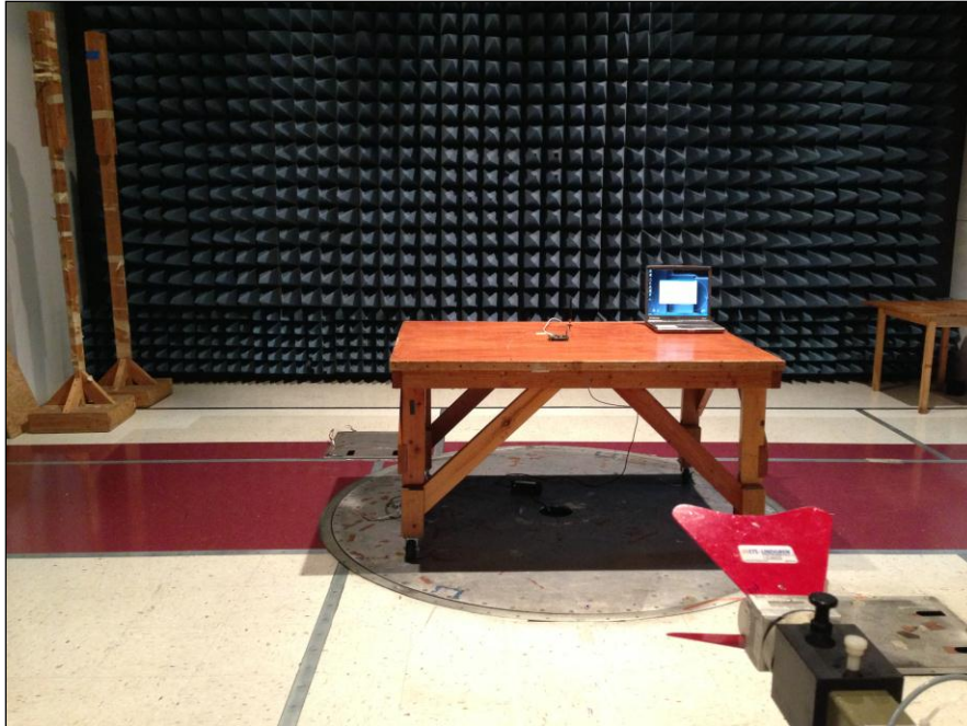
Photograph 9. Radiated Spurious Emissions, Test Setup, 3 m
