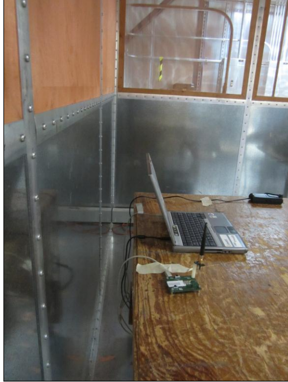
Photograph 7. Conducted Emissions, 15.207(a), Test Setup, Side View
