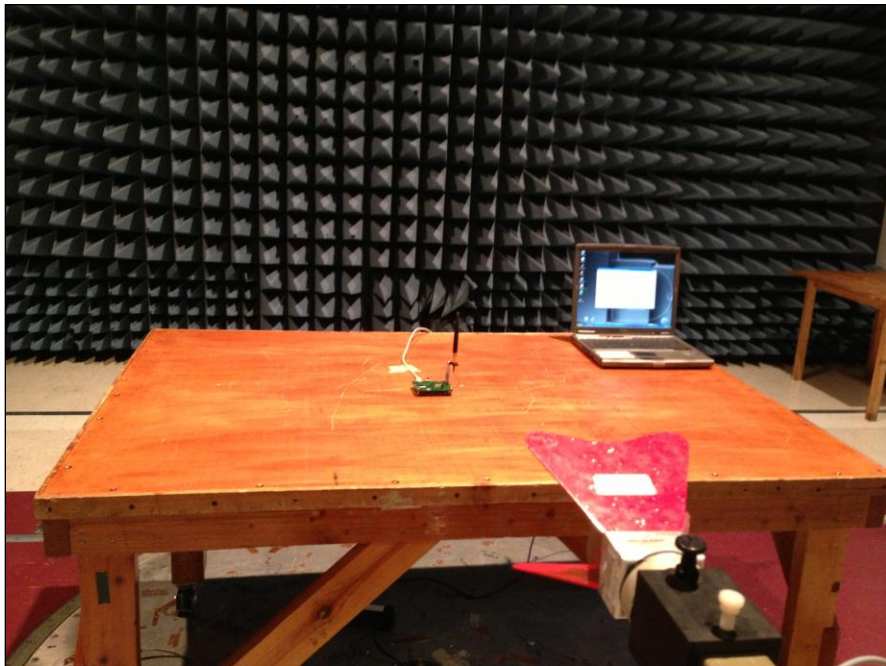
Photograph 8. Radiated Spurious Emissions, Test Setup, 1 m
