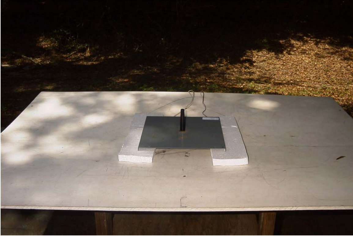
RADIATED EMISSIONS TEST SET UP WITH \frac{1}{4} WAVE ANTENNA-COAX ASSEMBLY, RFM PART NO. 500-1142-001
