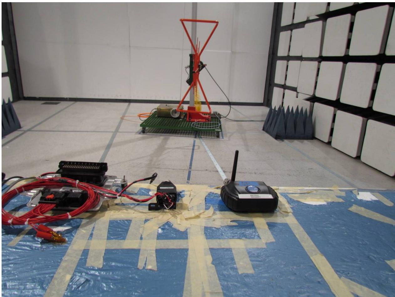
Receiver Radiated Emissions above 1 GHz
