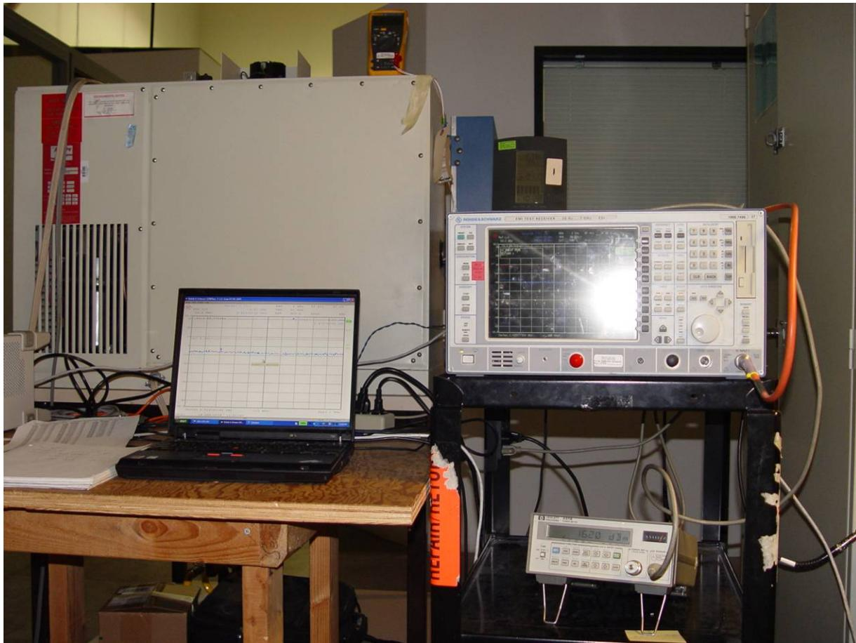
Conducted RF Emissions - Test Equipment
