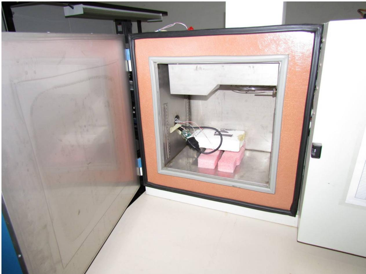
Transmitter Radiated Spurious Emission below 1 GHz
