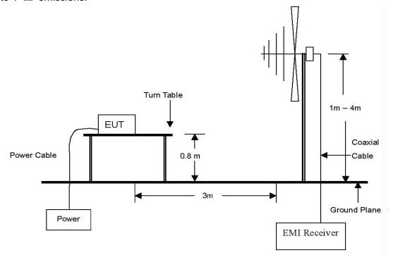
The diagram below shows the test setup that is utilized to make the measurements for emission from 1  $\oplus$  to 24  $\oplus$  emissions.
