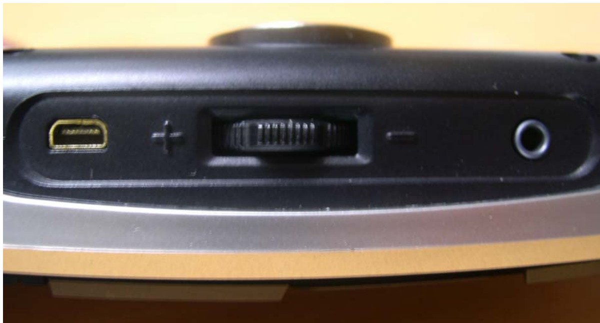
<Photograph 3: External Interface View> - USB Charging Port and Earphone Jack
