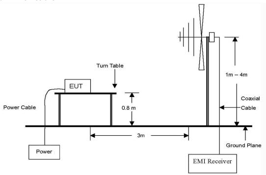
The diagram below shows the test setup that is utilized to make the measurements for emission from 1  $\times$  to 24  $\times$  emissions.
