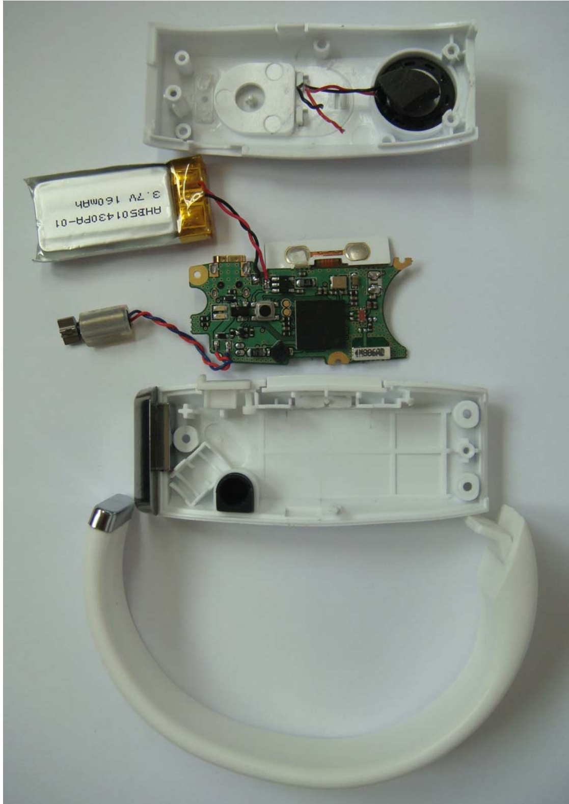
<Photograph 1: Cover removed>
