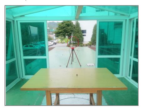
Photo of radiated spurious emission at 30 № ~ 1 000 №
