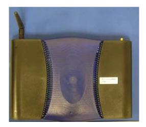
The radio utilizes a maximum gain of 3.0dBi dipole antenna. The Antenna connector used on this access point is a reverse polarity type of SMA connector
