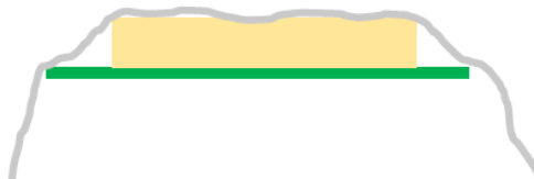
2) Antenna with PCBA and Silicone sheet (flat against antenna surface and draped over sides)
