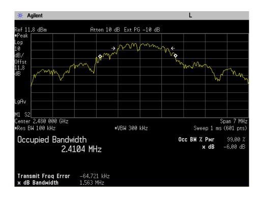
**Transmitter Power Spectral Density (PSD)**
