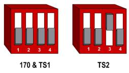
Figure B.2. SW1 settings for TS controller types (switch 3 only)
