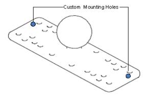
Figure 2.5. Factory installed ball plate (rectangular)
