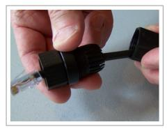
Figure 6.10. Thread cable through connector B
