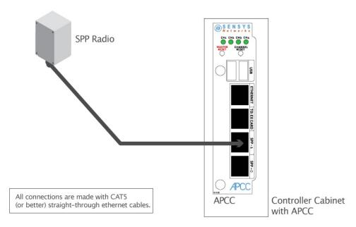
Figure 4.1. SPP radio powered from a traffic controller
