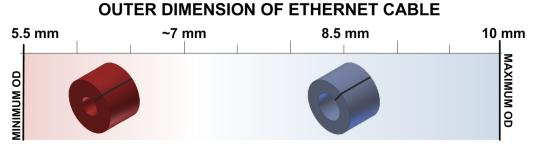
Figure 6.11. Ethernet cable bushing chart (not to scale)
