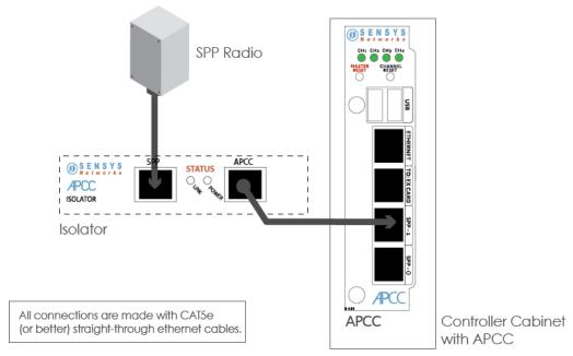
Figure 4.2. SPP radio powered from a traffic controller
