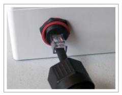
Figure 6.15. Connect cable to input jack
