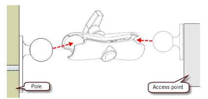
Figure 6.3. Double socket arm installation
