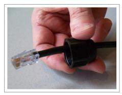
Figure 6.9. Thread cable through connector A
