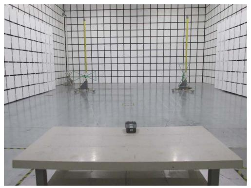
Description: Radiated Emission Test Setup for 1~18GHz
