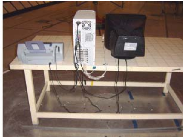
Test set up for radiated disturbance measurement
