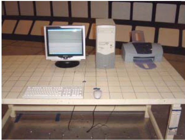
Test set up for radiated disturbance measurement
