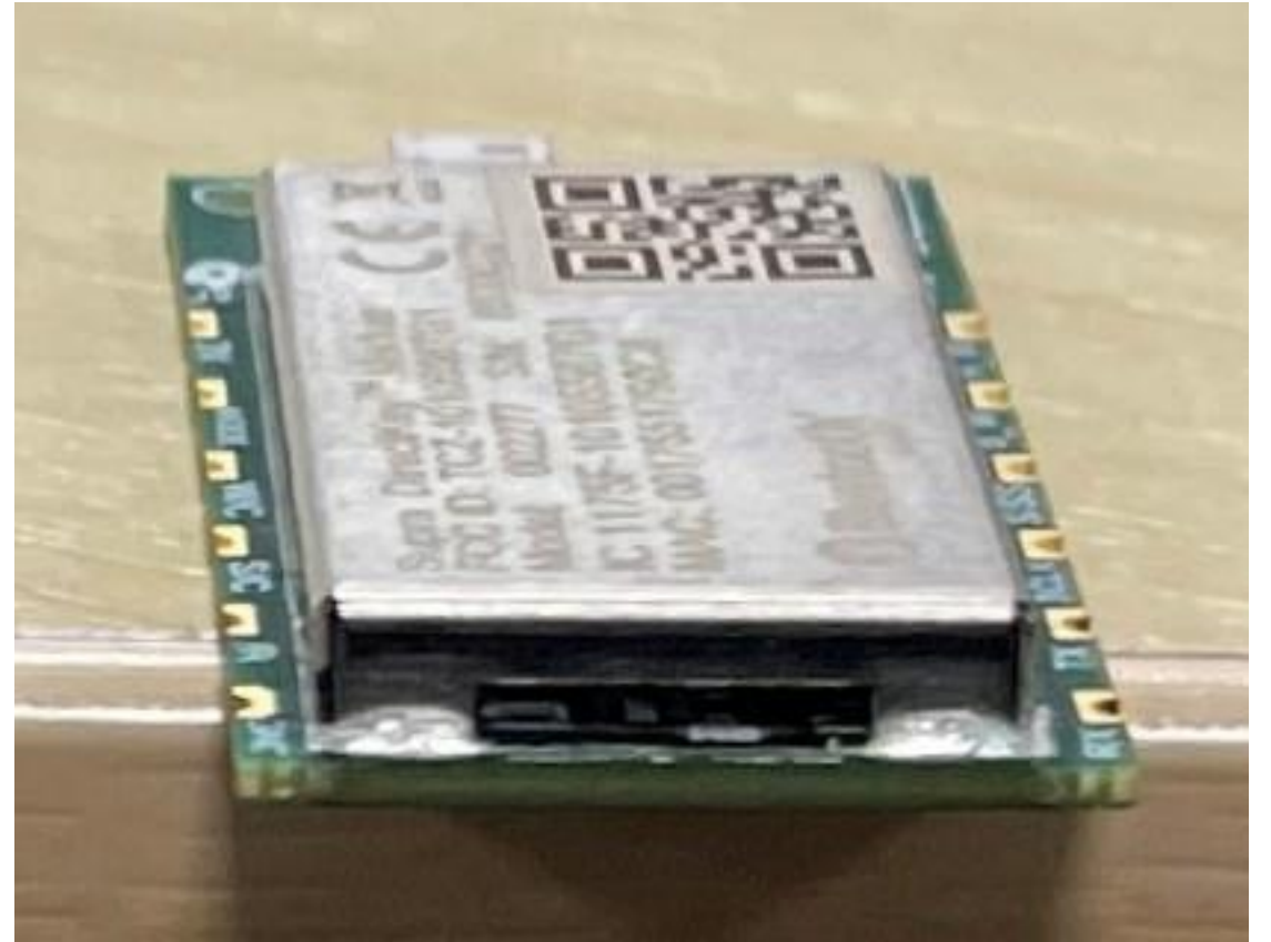
Side 4 with RF Shield
