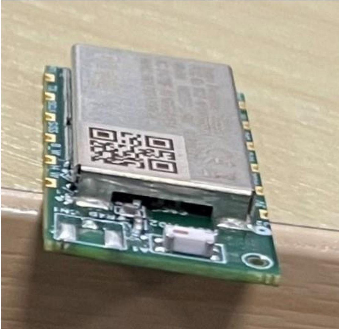
Side 3 with RF Shield
