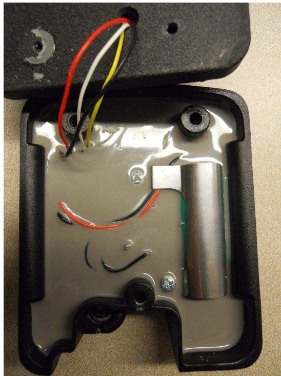
Inside Front Cover – picture shows completed assembly with potting material
