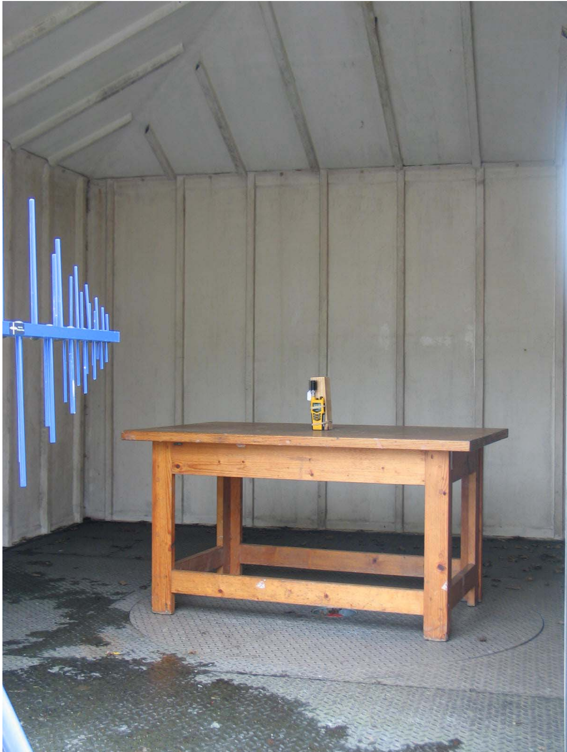
Photograph 2: Test setup radiated emissions (>30 MHz)
