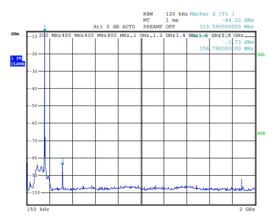
Note: to determine absolute values, the marker values in the plot must be compensated for 40 dB external attenuation.
