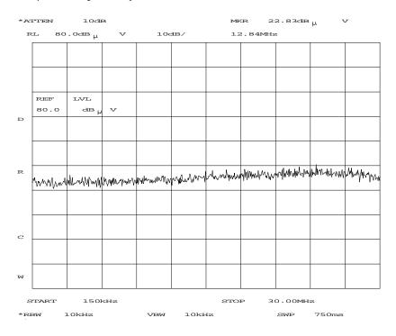
Remark: As no emissions above measuring system noise floor were detected, measurements on the Open Area Test Site were deemed not necessary.
