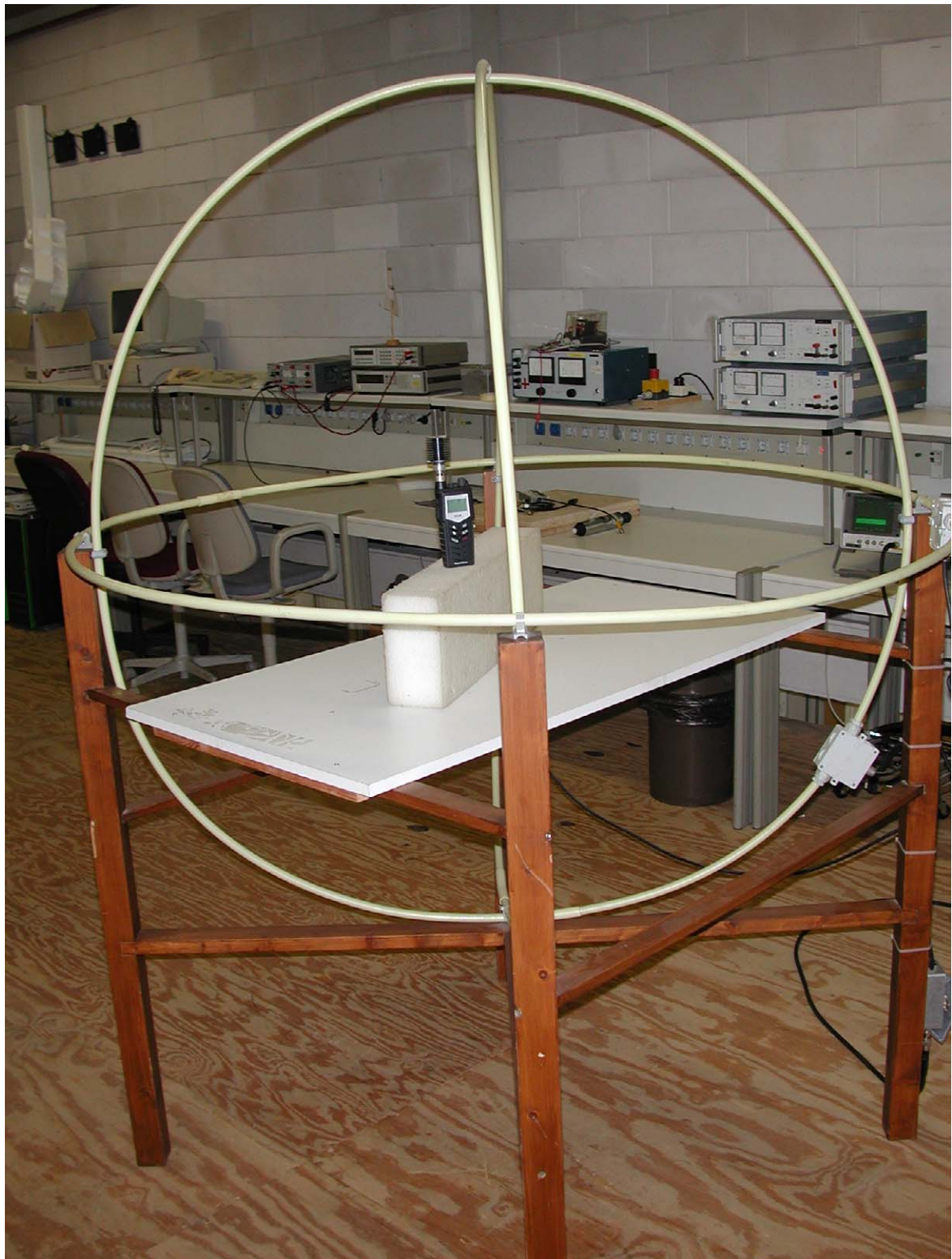
Photograph 1: Test setup radiated emissions (<30 MHz)
