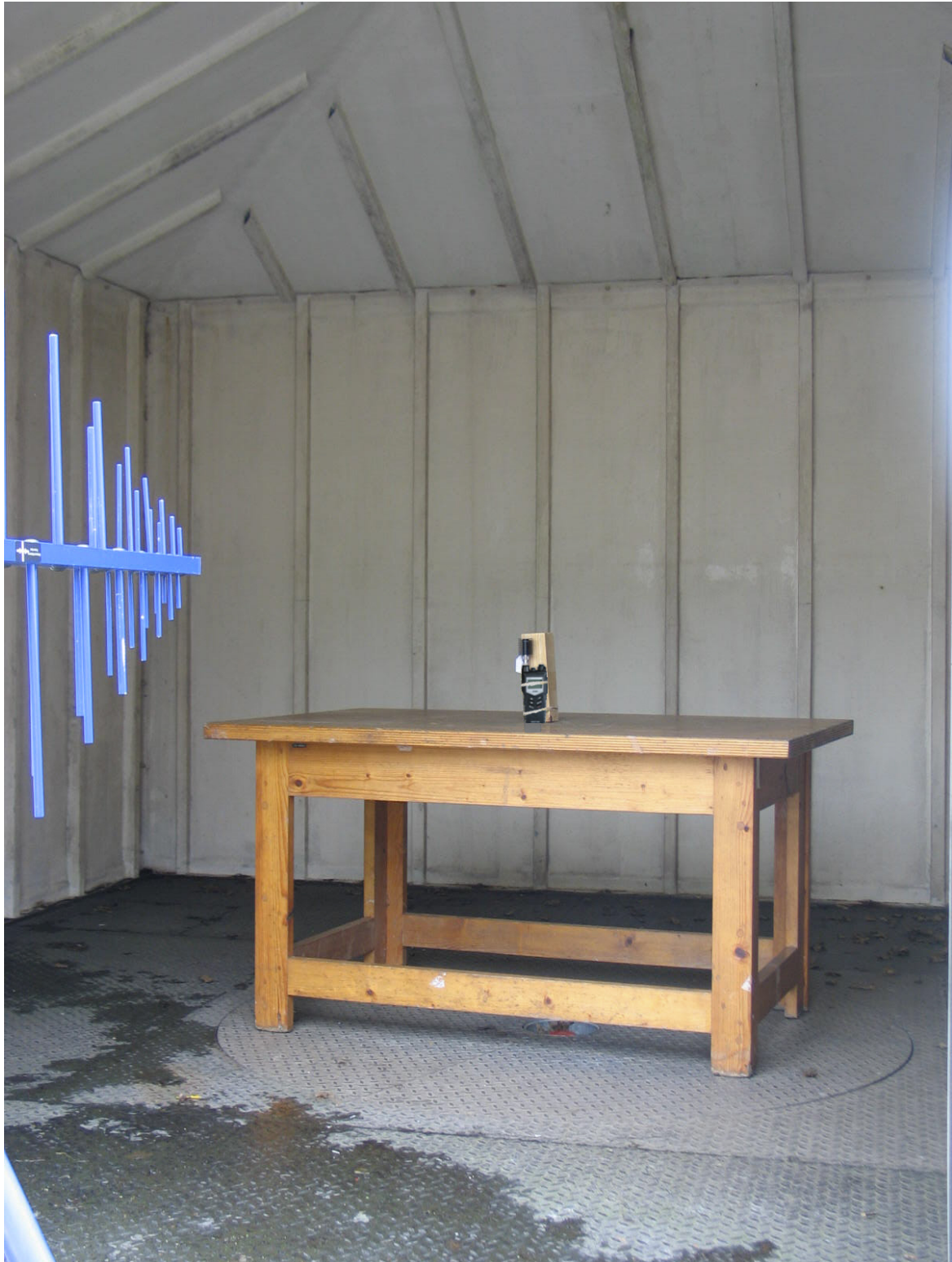
Photograph 2: Test setup radiated emissions (>30 MHz)
