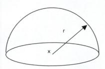
r = safety distance from the antenna placed at x emitting Rf radiation in an hemispherical pattern
