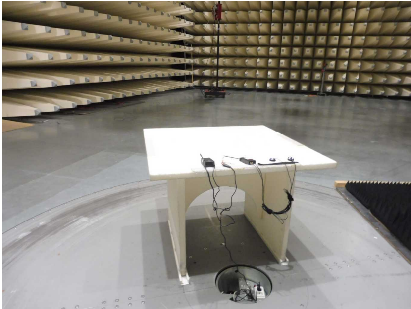
Photo 7: EUT at the semi-anechoic chamber
