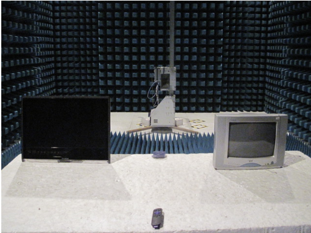
Description : Radiated Emission Test Setup for 1~18GHz
