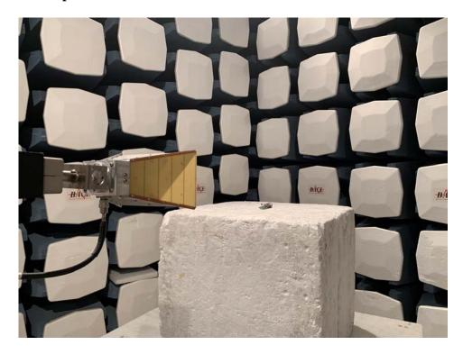
1.4 Radiated Spurious Emission 1-18 GHz Rear View
